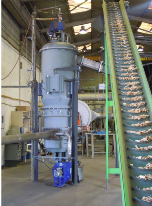
100 kW capacity Syngas from wood chips
