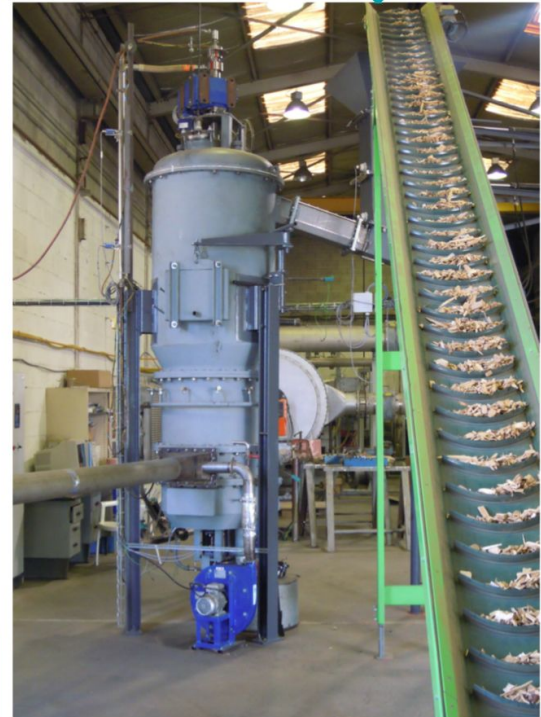
100 kW capacity Syngas from wood chips
